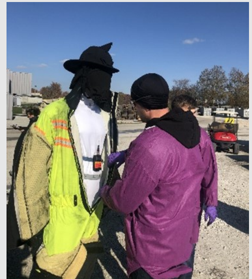
An IFSI Research team member dresses a mannequin in firefighting gear and attaches an air collection device under the firefighting personal protective equipment (PPE). The mannequin was placed in a smoke chamber so that the air collection device could record volatile organic compounds (VOCs).
